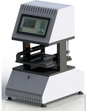
With this instrument it is possible to determine the bending strength, the fracture module, and the bending arrow of the sample by operating according to the Norms:
