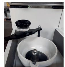
jar holder cup made of a single piece of casting
