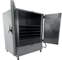
The temperature control is entrusted to a K1PX type microprocessor programmer with which it is possible to set and memorize drying cycles consisting of a maximum of 8 STEPS or to set a working temperature that will remain until it is changed.
